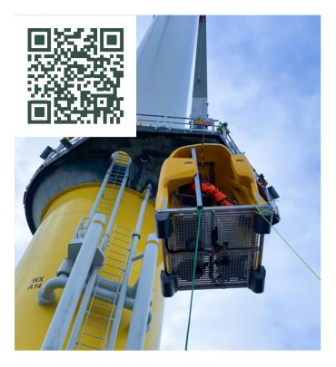
With Spider, technicians no longer need to climb the boat landing ladders to enter the transitions pieces (TPs), nor is it necessary to equip the TPs with separate lifting systems for personnel and cargo.
